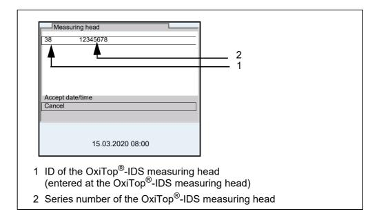
5 Using Accept date/time, confirm the date and time for the measuring head.
